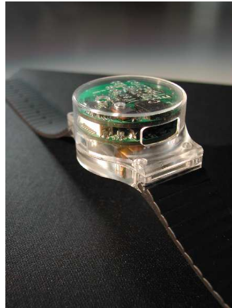
Fig. 3. The complete SensorButton and power supply, mounted as a wrist-worn unit
